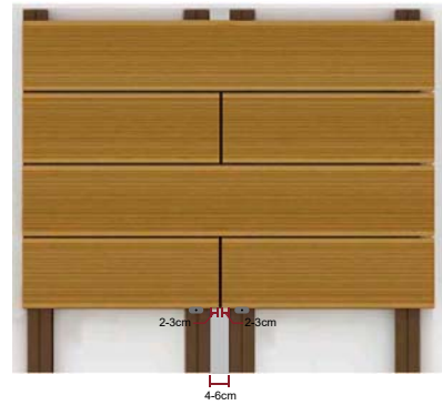
Staggered Installation Method
